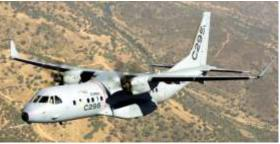
• The C-295MW is a transport aircraft of 5-10 tonne capacity and has a rear ramp door for quick reaction and para dropping of troops and cargo. It is powered by Pratt & Whitney PW127 engines, part of the PW100 family. All 56 aircraft will be installed with indigenous Electronic Warfare Suite.
